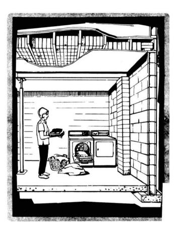
Protection is provided in a basement corner by bricks or concrete blocks between the overhead joists. A beam and jack column support the extra weight.
